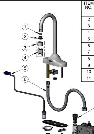
ITEM SALES NO. **DESCRIPTION** 006575-45 -015 O-Ring 044A 3/8" to Aerator Adapter B-0199-21-VRF VR 2.2 GPM Laminar Flow Device, 55/64-27 UN w/ Key 015425-45 Vandal Resistant Key 017195-45 Sensor Cable Assembly 016297-45 Inlet Hose, Faucet, 1/2" NPSM-F x 1/4" NPSM-F **EC-FILTER** Replacement Filter ChekPoint Control Module w/ Filter Tee 016647-45 5EF-0002 **AC Transformer** 5EF-0006 Temperature Mixing Valve 5EF-0005 Supply Hose. 9/16-24 Female x 1/2" NPSM
