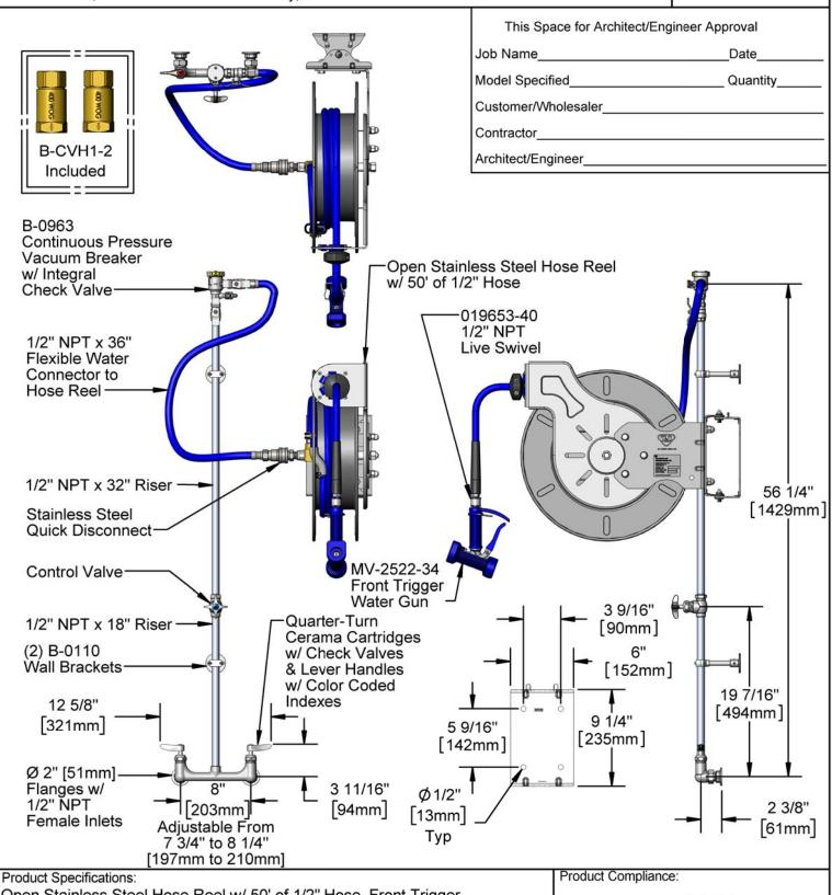
Open Stainless Steel Hose Reel w/ 50' of 1/2" Hose, Front Trigger Water Gun w/ Swivel, 1/2" NPT Vacuum Breaker, 1/2" NPT Flexible Water Connector, 8" Wall Mount Mixing Faucet, Control Valve, Horizontal Check Valves & EasyInstall Wall Swing Bracket
