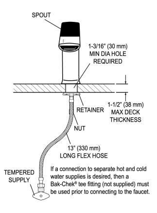
supply upon removal eliminating, need to access control stops. Solenoid carrier includes strainer for easy above deck service. Thermostatic mixer ordered separately to comply with ASSE 1070 requirements. The product shall be tested and certified to industry standards: ASME A112.18.1M, CSA B125.1, California Health and Safety Code 116875
