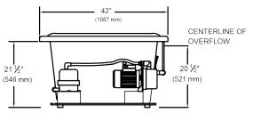
Installer Note: Due to the freeform shape of this tub, it is recommended that the tub be on the jobsite before making the final cut out for drop-in installation.
