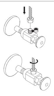
Install flex water supply lines on the angle stops and tighten with an adjustable wrench. Turn on both the cold and hot main valves
