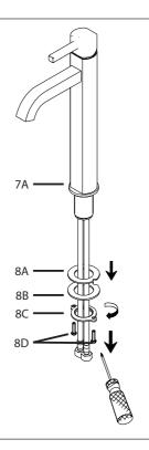
Remove rubber washer (8A), metal washer (8B), mounting nut (8C), and mounting screws (8D). Keep the base trim ring (7A) and rubber washer (7B) on the base of the faucet
