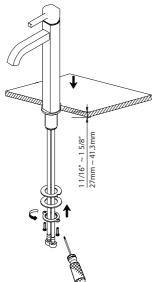
Install the faucet through the 1-3/8" predrilled hole in the countertop. Attach rubber washer (8A), metal washer (8B), mounting nut (8C), and mounting screws (8D) on the threaded mounting pipe. Tighten the mounting nut (8C) until snug. Tighten screws (8D) on the mounting nut (8C) with a Phillips head screw driver until snug
