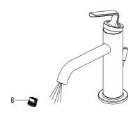
After installing faucet, remove aerator (B) with a coin. Turn water on for 30 seconds to remove any debris. Reassemble aerator (B).
