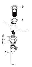
Insert drain flange (b) through drain hole with rubber washer (c) attached. From underneath, place concave (d) and metal washer (e) on drain flange. Secure with mounting nut (f). Thread tailpipe (g) onto drain (b) and hand tighten.
