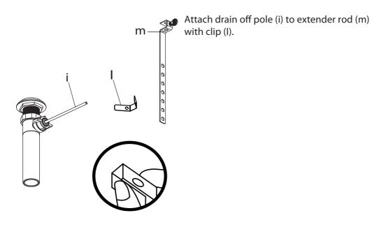
Step 3F: Installing the drain
