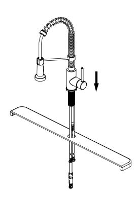
Optional No Escutcheon Installation. Insert faucet body through the hole in the sink.
