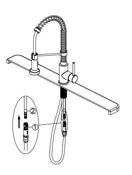
Push the quick connector (1) firmly upward and attach it to the receiving block (2). Pull down moderately to ensure the connection has been made.
