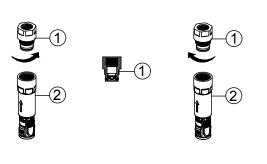
This faucet ships with a (WHITE) 1.8 GPM flow restrictor installed. An optional (BLACK) 2.2 GPM flow restrictor is also included in the box.
