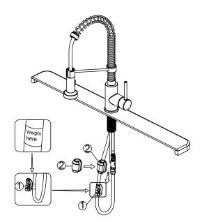
Install the weight clip (1) at the point of the hose marking "weight here". Insert the weight (2) onto the clip (1) by sliding it down onto the clip (1).
