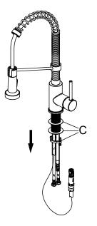
Shut off the water supply. Remove the old faucet. Clean the mounting surface. Remove mounting hardware (C) from faucet body (B).
