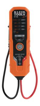
Klein Tools ET40 is an Electronic AC/DC Voltage Tester. It features indicators for positive and negative DC polarity, and tests DC voltages as low as 1.5V. It tests AC voltages 12-240VAC. Excellent for checking, verifying or troubleshooting common residential electrical wiring in electrical outlets, light fixtures, doorbells and more. It operates on 2 x AAA batteries.
