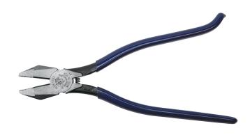
Twist and cut rebar tie wire with Klein Tools 9-1/4-Inch Ironworker's Pliers. They feature knurled jaws for a good grip and a spring-loaded design which enables self-opening. Unique handle tempering helps absorb the "snap" when cutting wire.
