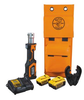
Klein's battery-operated Cable Crimper is engineered to make linemen's work more efficient by reducing the time and effort needed on the job. Crimps up to 600 MCM copper, 350 MCM aluminum and 477 ACSR cable. 7-ton hydraulic force crimps a larger capacity faster than similar models on the market. Compatible with industry standard W-style dies. Powered by a DeWALT 20V lithium-ion battery (4 Ah). Includes cutting jaw, two 4 Ah batteries, charger and bag.
