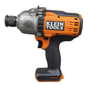
For professional impact fastening and drilling applications. With up to 500 foot pounds of max torque, the impact wrench is great for drilling using auger bits and driving fasteners into wood, metal and concrete. It features a variable speed trigger and 7/16" quick release chuck.
