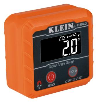
The Klein Tools Digital Angle Gauge and Level can measure or set angles, check relative angles, or can be used as a digital level. The strong magnetic base attaches to ferromagnetic surfaces such as conduit. Along with dual measurement ranges of 0 to 90-Degree and 0 to 180-Degree, this tool has a high visibility reverse contrast display for easy viewing.
