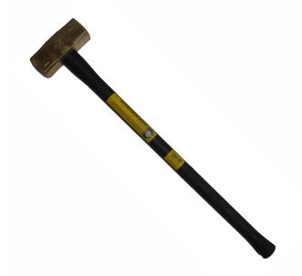
This Sledge Hammer from Klein Tools features a brass head designed for use in non-sparking environments. The brass head also provides a softer, non-damaging blow. The comfortable, thick rubber grip handle provides better protection from shock and vibration.
