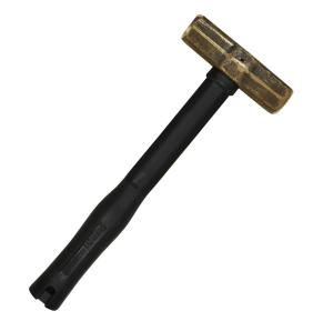
This Sledge Hammer from Klein Tools features a brass head designed for use in non-sparking environments. The brass head also provides a softer, non-damaging blow. The comfortable, thick rubber grip handle provides better protection from shock and vibration.
