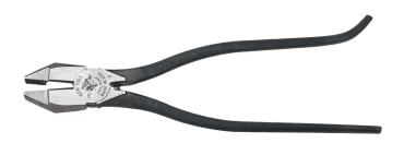
Use the Klein Tools Ironworker's Work Pliers to twist and snip soft annealed rebar tire wire. The knurled jaws also aid in easy twisting and turning. These pliers feature a hook-bend in the handle for added grip and leverage. Unique handle tempering helps absorb the "snap" when cutting wire.
