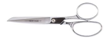
Industrial quality trimmers hold a keen edge even when switching from fine fabrics to heavier material. Cut fabric, canvas, felt, lining, silk, muslin, cord and almost any other material in the textile industry. Hot drop forged, Chrome over nickel plated. 7-1/2-Inch (190.5 mm) overall length. 3-1/2-Inch (88.9 mm) cut length.
