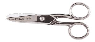
The 100CS is nickel plated with wire stripping notches for 19 and 23 gauge wire. Blades hardened to 59 to 61C Rockwell for extra cutting life with serrations for holding wire while it cuts.
