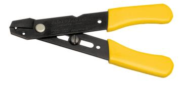
A handy, light, compact tool for stripping 12-26 AWG solid and 14-28 AWG stranded wire. Features convenient hole for looping or bending wire. Adjustable slide stop with set screw for repeat stripping work.
