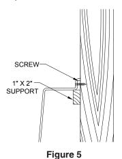
Carefully drill 1/8" holes through the tile flange at each stud location.
