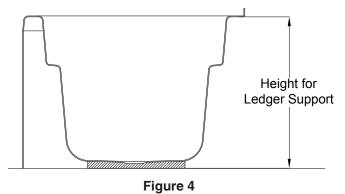
Install the 1" x 2" support ledger strip to the framing to allow support along the entire rear ledge of the bath (see **Figures 2 and 5**).
