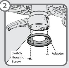
Using the switch housing screws that you removed from the cap, install the adapter.
