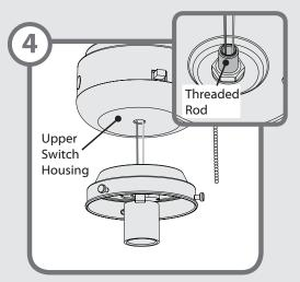
Lift the light kit up, tucking the wires into the hole in the switch housing. Install the center stem of the light kit into the lower switch housing by turning the threaded rod clockwise into the threaded hole. Continue turning until tight.
