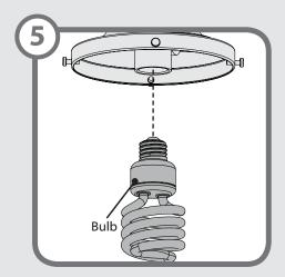
Install a bulb into each of the sockets. When necessary, replace with bulbs of the same wattage.
