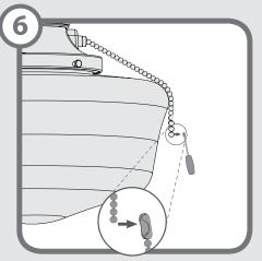
Installing the pull chain pendant -Attach the pull chain pendant to the end of the short chains coming from the switch housing and the light kit.
