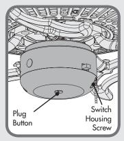
If your fan's switch housing cap resembles this one, remove the whole switch housing by removing the switch housing screws with a Phillips head screwdriver. Remove the plug button using a standard screwdriver. Then follow the **TYPE-D ASSEMBLY INSTRUCTIONS** on pages 10-11.
