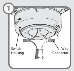
If your fan does not have pin connectors on the wires coming from the switch housing, install the wiring harness provided. Using the provided wire connectors connect the white wire from the fan to the white wire from the wire harness and connect the black or blue wire from the fan to the black wire from the wire harness.
