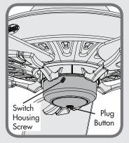
If your fan's switch housing cap resembles this one, remove the whole switch housing by removing the switch housing screws with a Phillips head screwdriver. Remove the plug button. Then follow the **TYPE-C ASSEMBLY INSTRUCTIONS** on pages 8-9.
