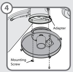
Lift the light kit up to meet the lower switch housing. Using the mounting screws found in the hardware bag, install the light kit to the adapter.
