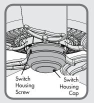
If your fan's switch housing cap resembles this one, remove the whole switch housing by removing the switch housing screws with a Phillips head screwdriver. Remove the two cap screws from the inside of the switch housing. Reinstall the switch housing. Tighten the switch housing screws. Then follow the **TYPE-B ASSEMBLY INSTRUCTIONS** on pages 6-7.
