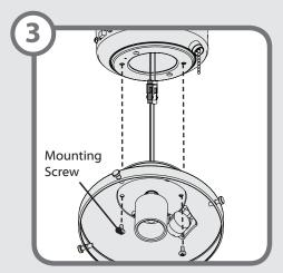
Lift the light kit up to meet the lower switch housing. Using the mounting screws found in the hardware bag, install the light kit to the adapter.
