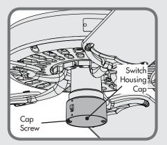
If you are installing this light kit onto a Hunter Original, remove the cap screws with a Phillips head screwdriver. Keep the screws Remove the cap. Then follow the **TYPE-A ASSEMBLY INSTRUCTIONS** on pages 4-5.
