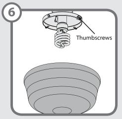
Installing the globe - To install the globe, first loosen the thumbscrews. Raise the globe to the light fixture. Tighten all thumbscrews securely.
