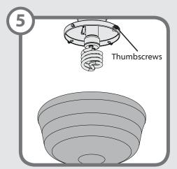
Installing the globe - To install the globe, first loosen the thumbscrews. Raise the globe to the light fixture. Tighten all thumbscrews securely.
