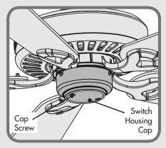
If your fan's switch housing cap resembles this one, remove the cap screws with a Phillips head screwdriver. Then follow the **TYPE-B ASSEMBLY INSTRUCTIONS** on pages 6-7.
