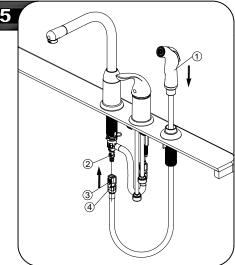
Insert side spray hose (1) through hose guide and sink. Align block (2) and tabs (3) on quick connect (4). Push quick connect housing firmly upward and snap onto receiving block. Pull down moderately to ensure connection has been made. If it is necessary to remove quick connect, squeeze tabs on hose between index finger and thumb, then pull down to disconnect.
