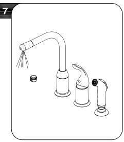
Important: After installation is completed, remove aerator assembly. Turn on hot and cold water supplies. Turn handle to full open position for one minute. Check for leaks. Replace aerator.
