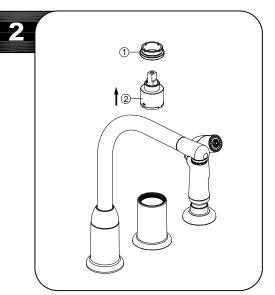
Loosen cartridge nut (1) by turning it counter-clockwise and lift out the cartridge (2).Insert new cartridge and retighten the cartridge nut. Reinstall the handle
