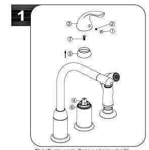
Shut off water supply. Remove set screw plug (1). With valves in "closed" position, unscrew set screw (2) and remove handle (3) from valve stem (4). Loosen the screw (7) from valve stem (4). Loosen the cap (5) from the cartridge nut (6).
