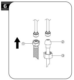
Make connections to water lines. Use 1/2" I.P.S. faucet connections (1) or use coupling nuts (3) with 3/8" O.D.ball-nose riser (2).Use wrenches to tighten connections.
