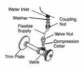
Connect the cold water supply line (not supplied) to the tank with your straight or angled stop. Place the washer, and then attach the plastic nut to the tank water inlet. If necessary, slightly bend the pipe to fit into the inlet hole on the water inlet. Tighten all plastic nuts securely.
