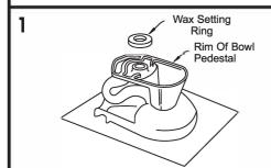
Clean the immediate floor area thoroughly. Insert the new toilet bolts in the slotted flange, bolt heads down. The toilet bowl should be placed on the floor upside down, on a soft material to prevent scratching. Place the wax ring evenly around waste flange (horn), with tapered end of the ring facing the toilet. Apply a thin bead of sealant around the toilet base.
