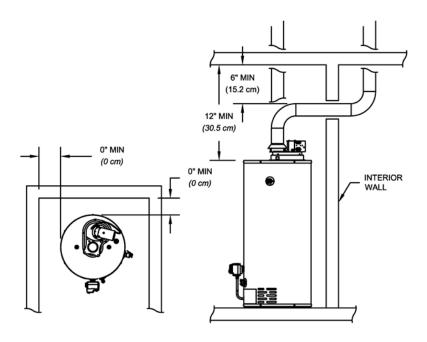
Figure 1. Minimum Clearances for an Alcove Installation.
