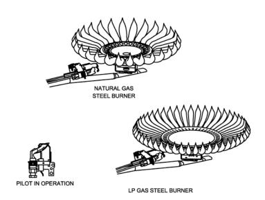
Figure 3. Burner and Pilot Assembly Used.
