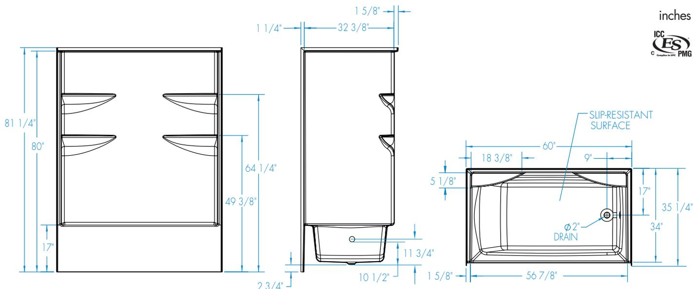
**FEATURES** lbs Dimensional Tolerance  $\pm 3/8"$ . Dimensions needed for site preparation should be measured from the unit. Aquatic assumes no responsibility for preparatory work.
